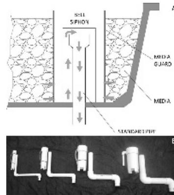
Figure 4. Bell siphon schematic (A) and examples of bell siphon (B) (12)
