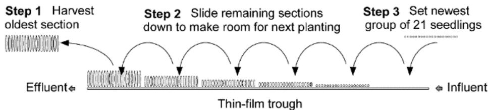
Figure 5. Schematic of a conveyor production system (CPS) (2)
